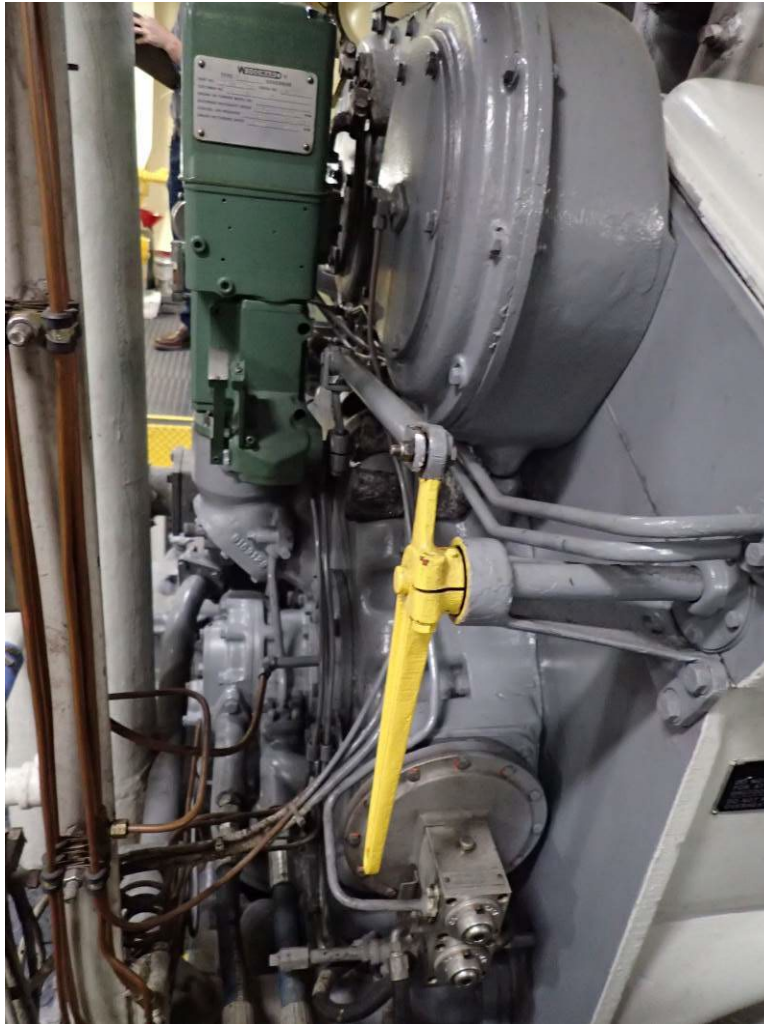
Photograph 66. - "B" Engine Governor and Linkages - Engine Idling
