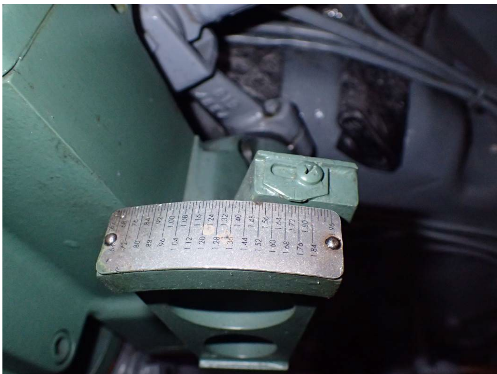
Photograph 70. - "B" Engine Governor Position - Engine Idling
