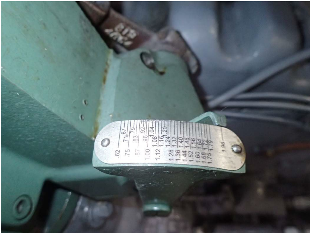
Photograph 54. - "A" Engine Governor Position - Engine Stopped
