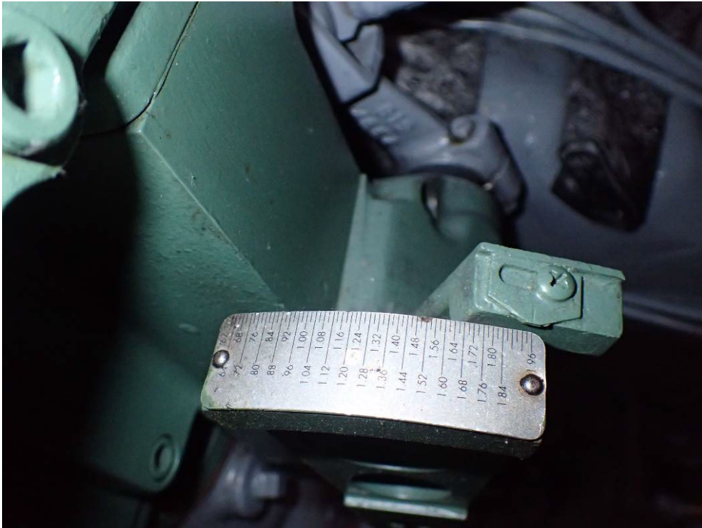
Photograph 43. - "B" Engine Governor Position - Engine Stopped
