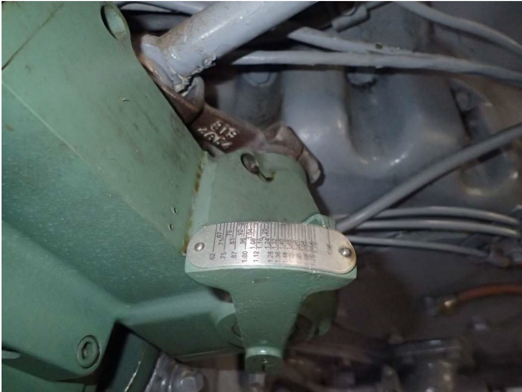
Photograph 53. - "A" Engine Governor Position - Engine Stopped
