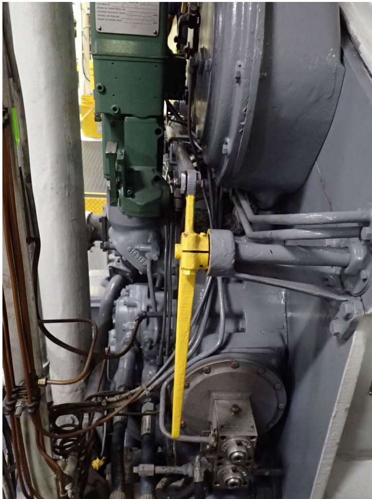
Photograph 44. - "B" Engine Governor and Linkages
