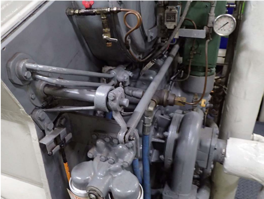
Photograph 49. - "B" Engine Governor and Linkages
