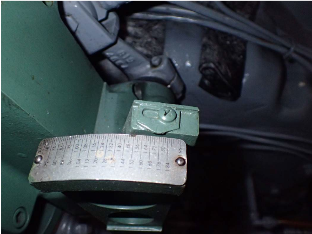
Photograph 71. - "B" Engine Governor Position - Engine Idling
