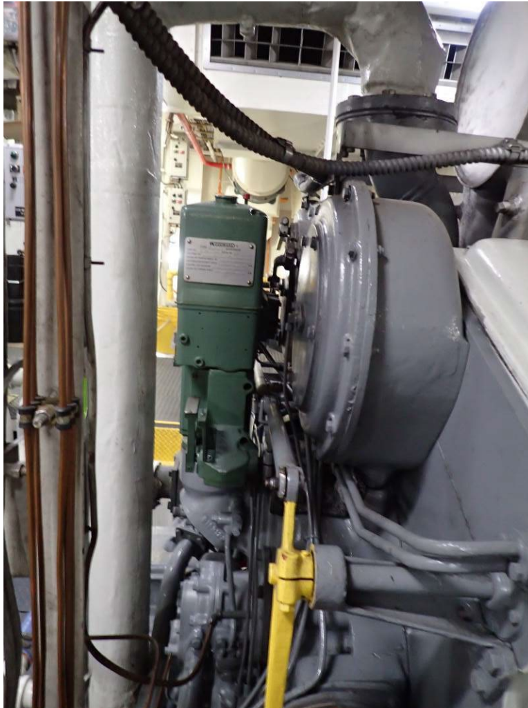
Photograph 40. - "B" Engine Governor and Linkages
