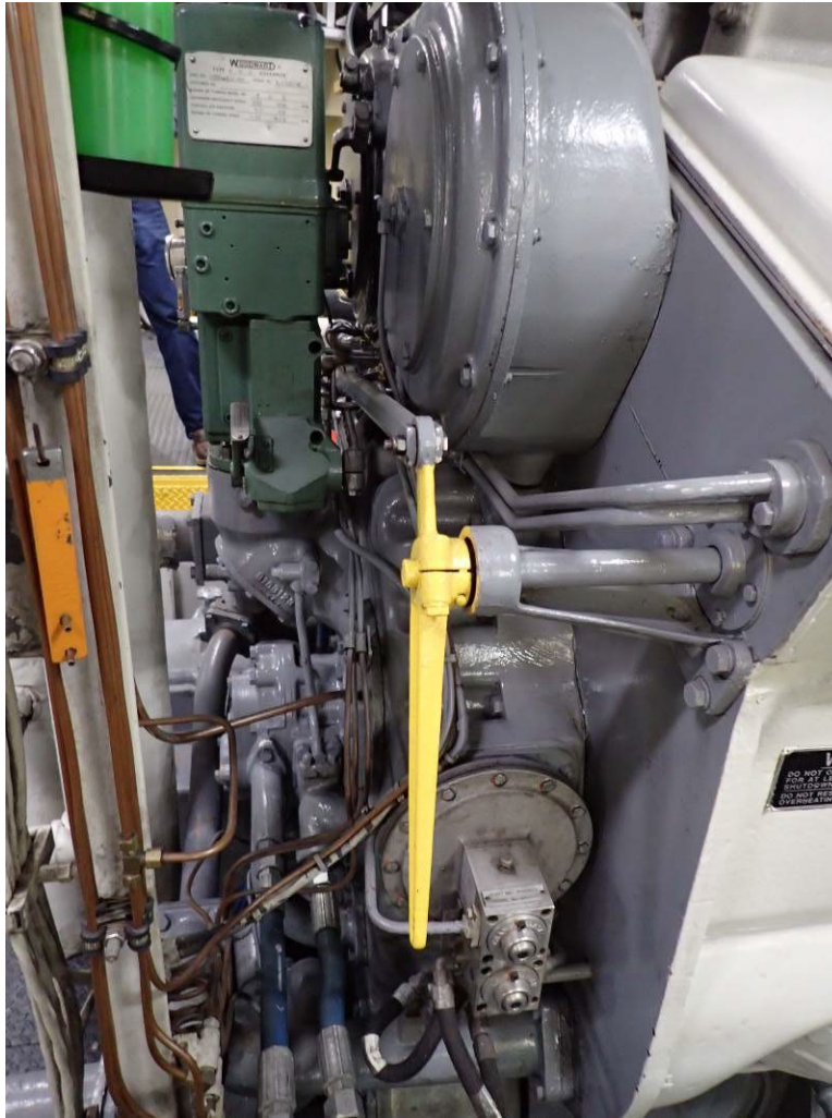
Photograph 52. - "A" Engine Governor and Linkages
