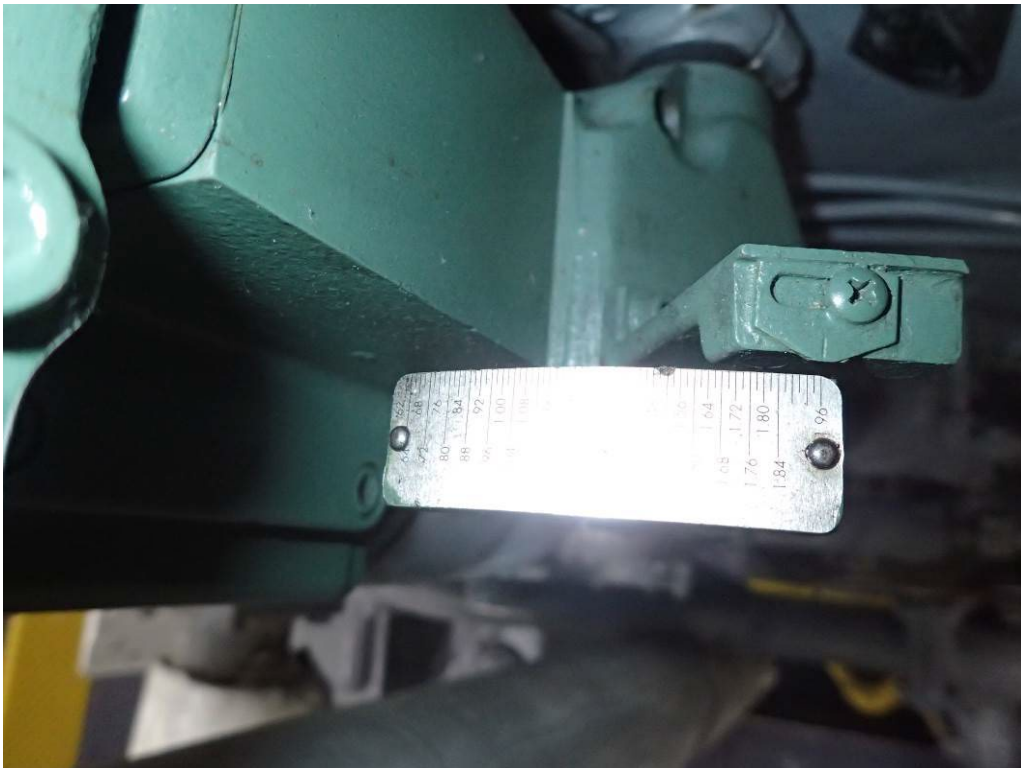
Photograph 42. - "B" Engine Governor Position - Engine Stopped
