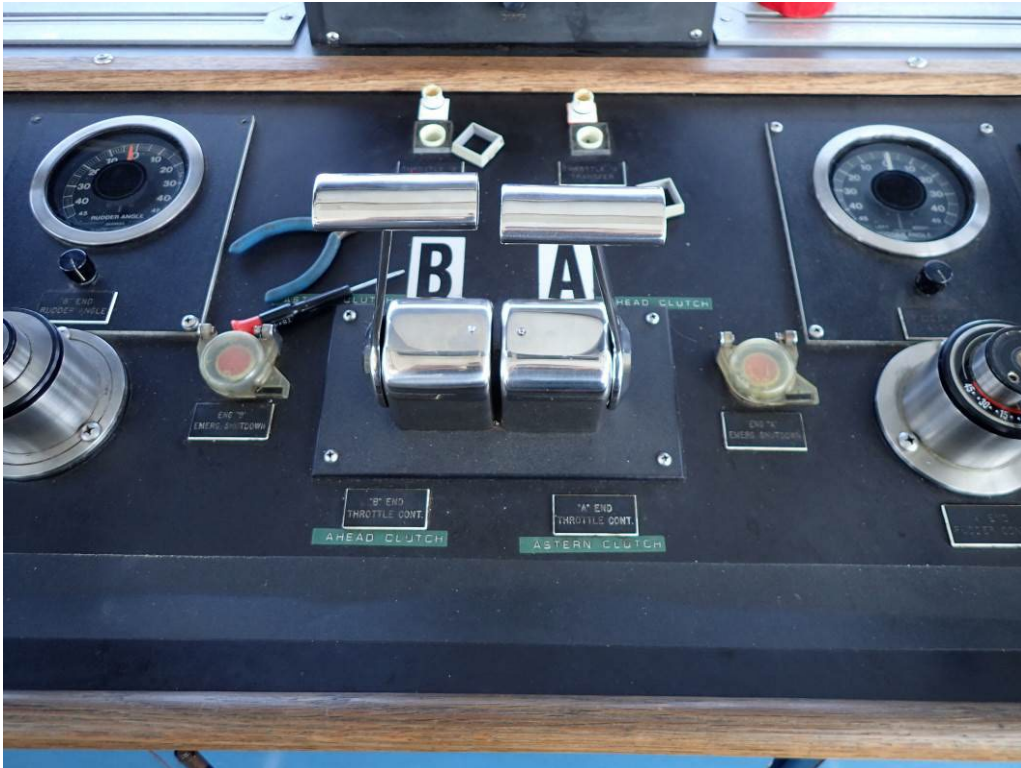
Photograph 3. - Ft. George-Facing/"B" End Clutch and Throttle Controls
